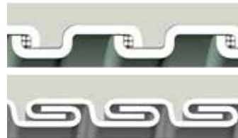
Square-Locked Design with cord packing 3/8" - 1-1/4"
